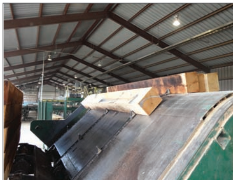
As with most tie plants, ties are loaded onto the chain for grading...
