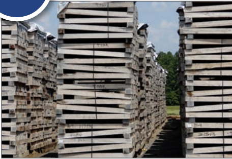
These ties were air-stacked in 2012 and rest side by side with those more recently stacked.
