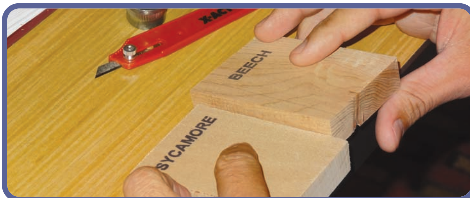
Inspectors may be called upon to distinguish between oaks and mixed hardwoods depending on how their railroad customer specifies their orders.
